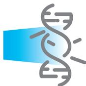
Exposure to UV-C light breaks down cell walls, reaches the cell's DNA and RNA, initially inactivating the cell from multiplying. With increased exposure, light continues to break down the organic material, destroying the cell entirely.
